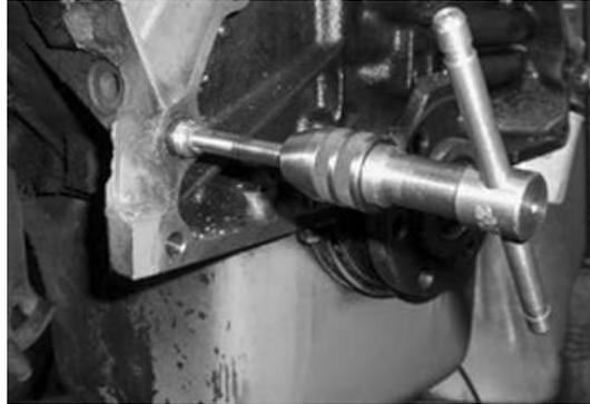
Alternatively, using a die it is possible to thread the pin and using nut or a slide hammer with a female thread adapter, pry the pin out. Take care not to ding or damage the bellhousing mounting face.
