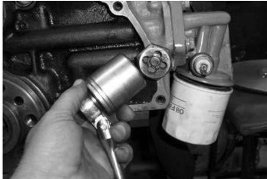
2. With the original locating pins removed, clean the pin holes and apply a light film of oil in the hole. Using care not to damage the hex in the head of the pin, carefully drive the pin into the block to the depth of the relief between the upper and lower portion of the pin.
