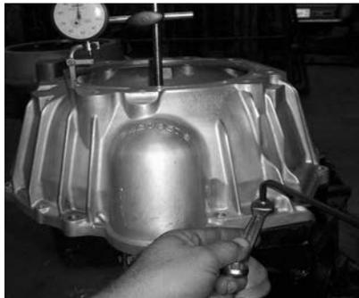
7. Loosen the bellhousing bolts in the same pattern as they were tightened only to the point where the bellhousing can be moved using the Allen wrench and open end wrench on the locating pins.
